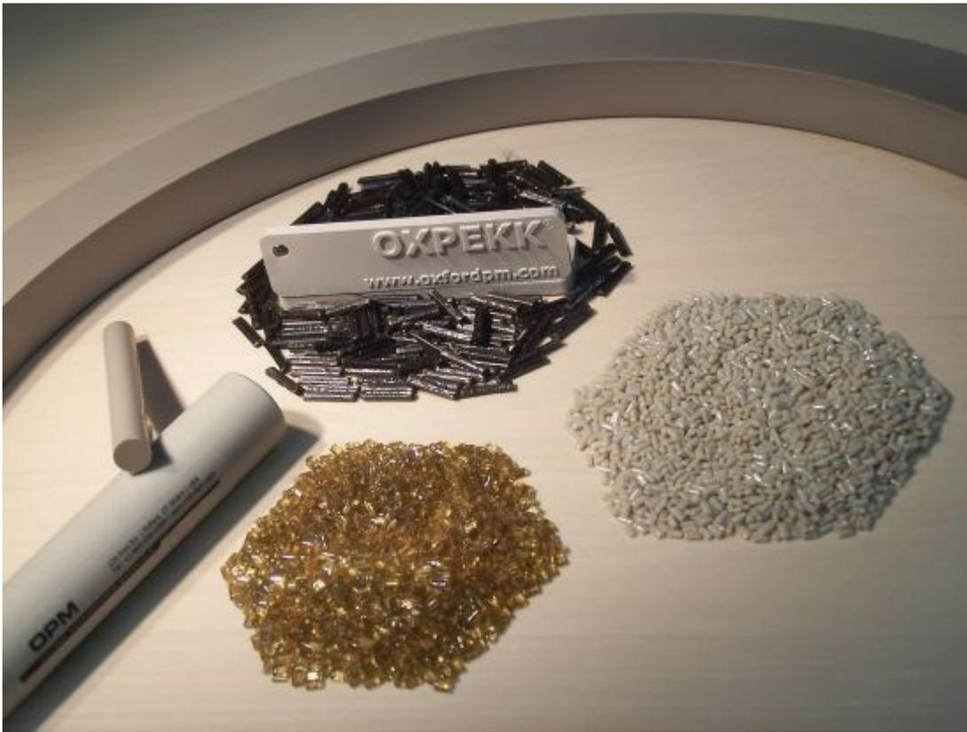
*OXPEKK is available in unreinforced pellets and rods as well as custom filled compounds, including carbon, glass and others. SOURCE: Oxford Performance Materials.*
